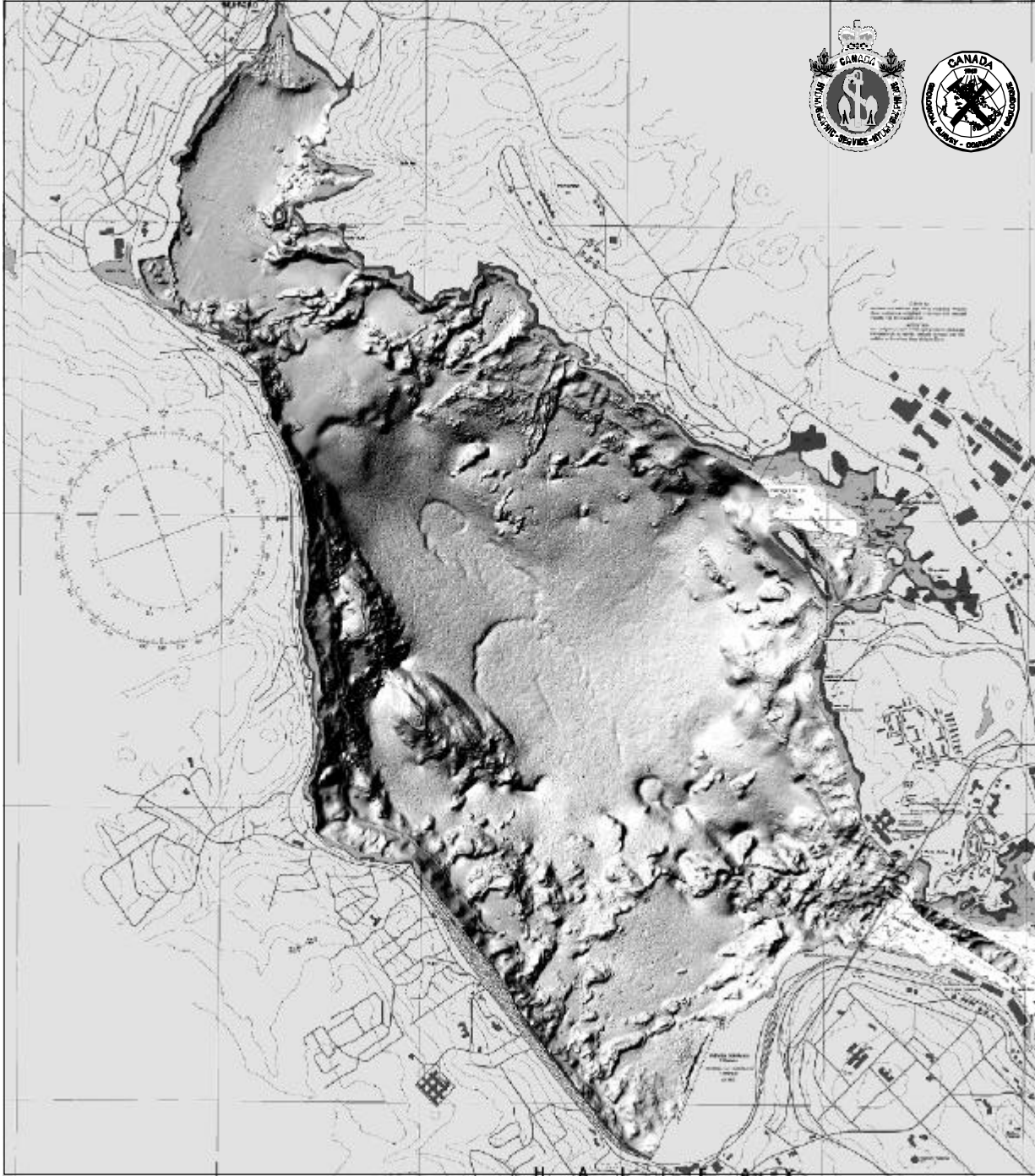
Figure 5: A shaded-relief, black and white multibeam bathymetric image of Bedford Basin (Fader et al., 2000b). Prominent features include boulder berms ringing the basin at 23m water depth, anchor marks, shipwrecks, subsidence depressions in deep water, and areas of bedrock outcrop. A benthic habitat assessment sampling program can be based on this information and other interpreted maps of seabed character.
