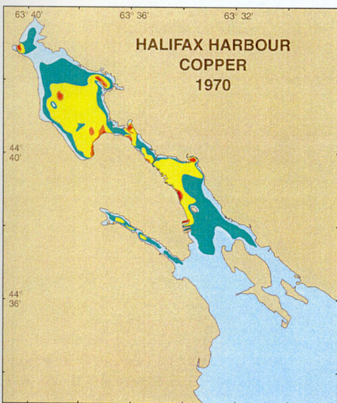
Figure 3. Copper in sediments of Halifax Harbour as measured in dated sediment cores.
