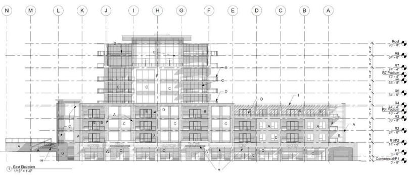
A - Masonry Type 1 - Red/Brown Tone B - Fibre Cement Siding - Light Beige Tone
