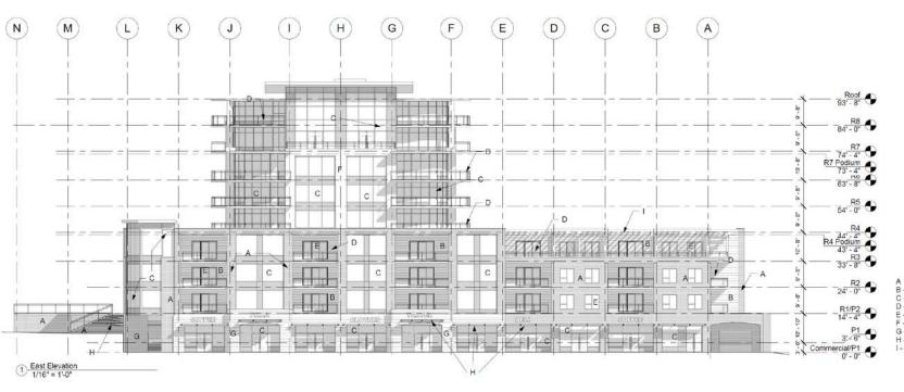
A - Masonry Type 1 - Red/Brown Tone B - Fibre Cement Siding - Light Beige Tone C - Aluminum Glazing System D - Aluminum/Glass Railing E - Virnyl Window/Door F - Fibre Cement Panel - Off White Tone G - Masonry Type 2 - Mid Beige Tone H - Aluminum/Glass Canopy I - Pergola - Brownish Tone
