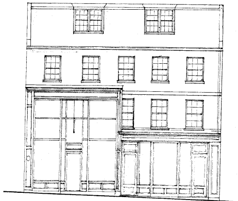
Sketch from Appendix A of Attachment G, showing 1906 enlargement of the old Hagarty storefront to create a two-storey display window for Barnstead's Drug Store. Enlarged storefront cuts through centre window on 2 nd floor. Windows changed to 6-over-6. Mansard roof and dormers were added in 1922.
