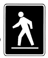
lane(s) with the pedestrian symbol oriented to the center of the roadway. As well as helping to indicate the location of the crosswalk at night, the illuminated RA-5 sign provides down-lighting over the crosswalk area.
