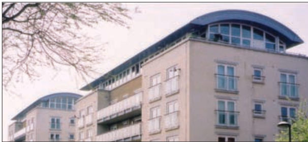
Rooftop elements such as mechanical rooms, elevator caps and stairway exits should be consolidated into a single structure, the design of which relates to the design of the overall building
