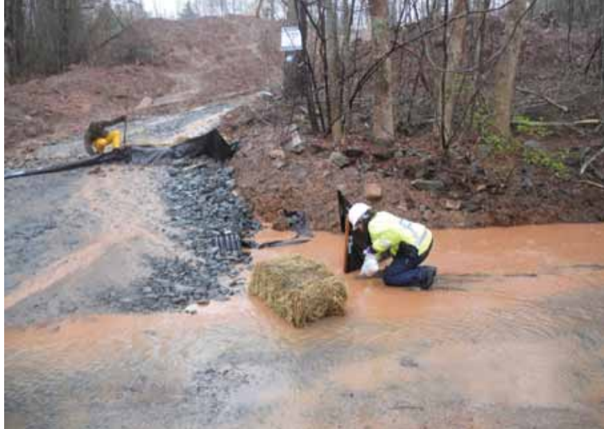
Environmental Services staff sample run off from a construction site
