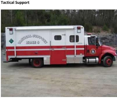
Tactical support trucks carry specialized equipment to the incident scene such as additional breathing apparatus air tanks and HAZMAT equipment.
