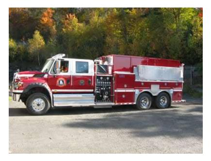
A tanker truck's primary purpose is to transport large amounts of water to the fireground to make it available for extinguishing operations. These apparatus are especially useful in rural areas where fire hydrants are not readily available and natural water resources are insufficient or difficult to exploit.
