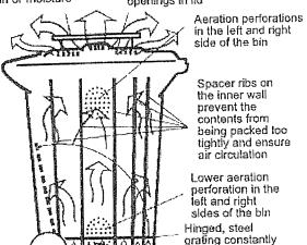
Spacer ribs on the inner wall prevent the contents from being packed loo tightly and ensure air circulation
