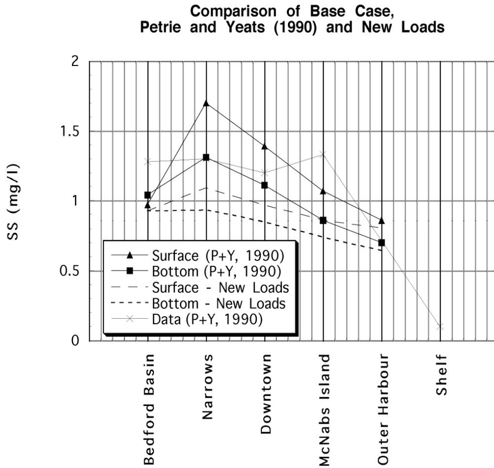
Figure 2.2 Suspended solids data comparison.
