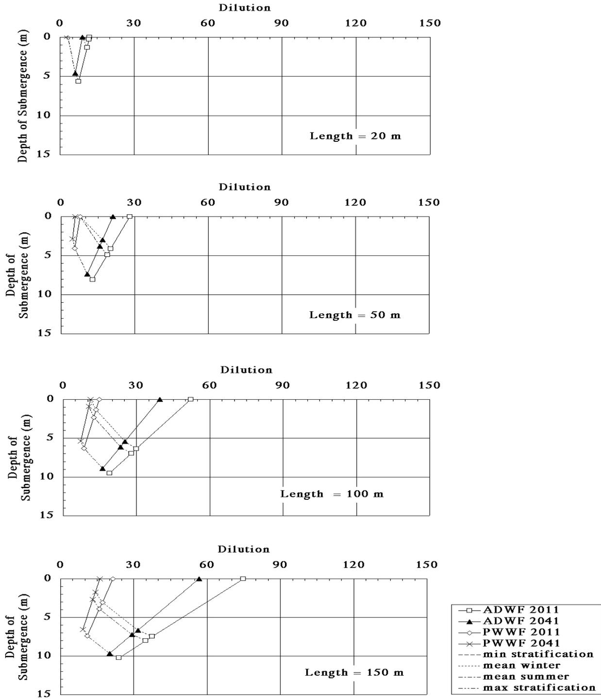
Figure 4.4 Diffuser analysis results - Site 2b.
