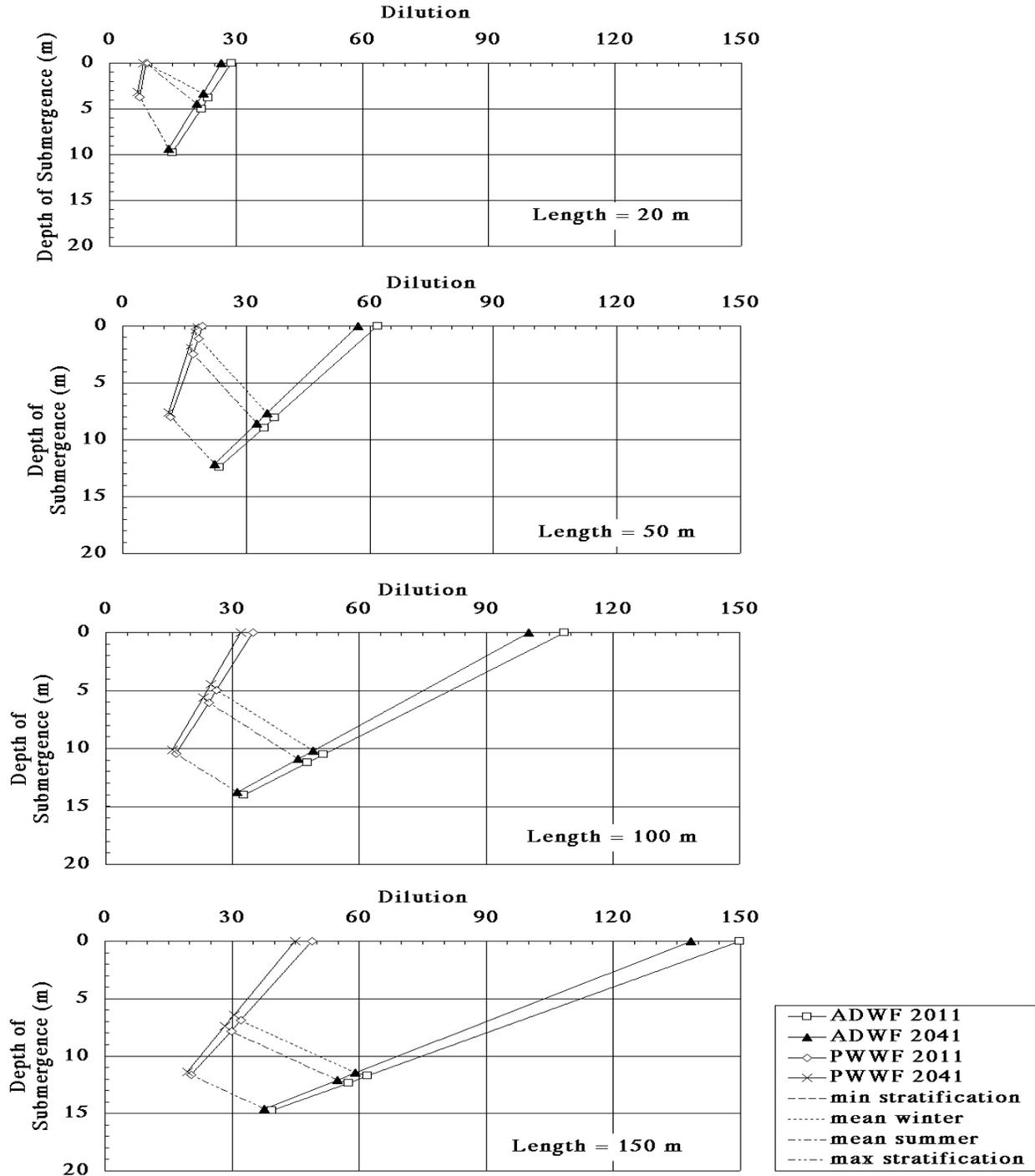
Figure 4.1 Diffuser analysis results - Site 1a.
