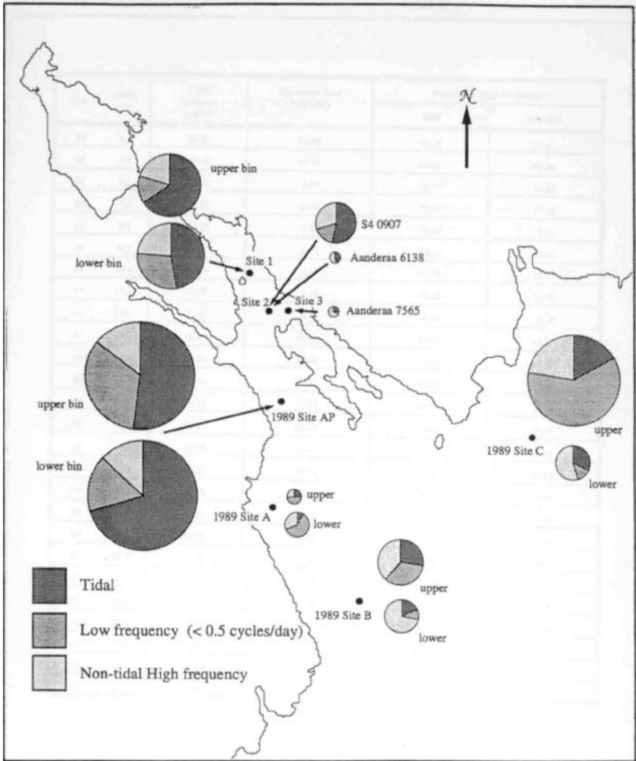
Figure 3.3 Observed currents in Halifax Harbour - Source: ASA 1990.
