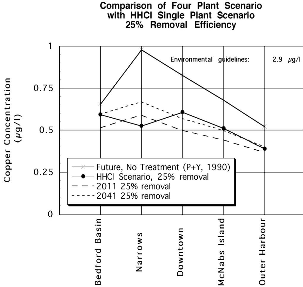
Figure 2.5 Predicted Copper levels with 25% assumed removal.
