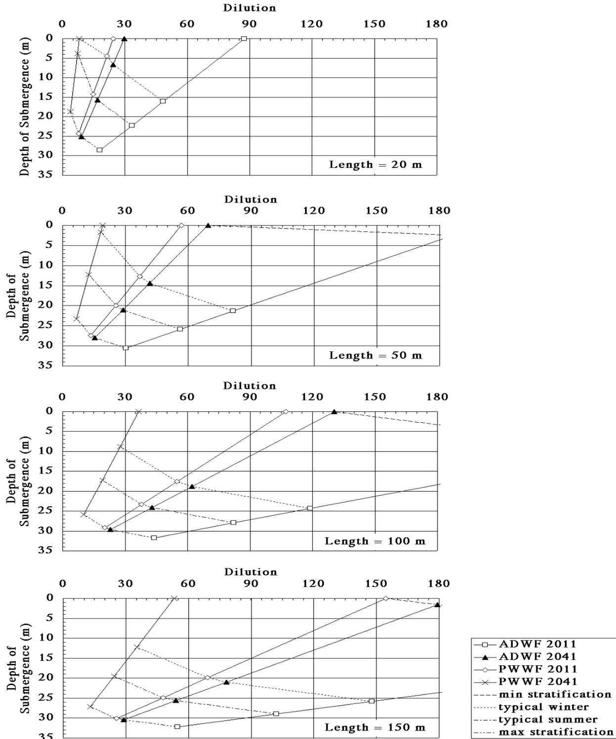
Figure 4.7 Diffuser analysis results - Site 4a.
