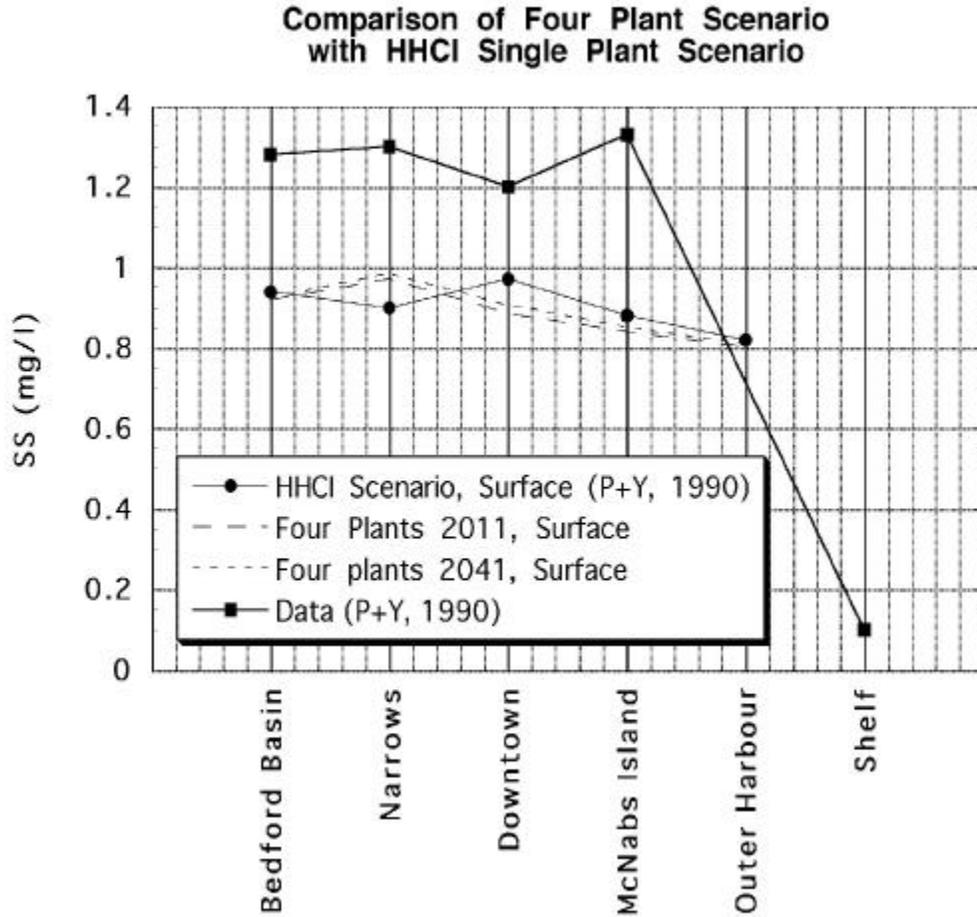
Figure 2.3 Predicted suspended solids - comparison of four plant and older one plant results.
