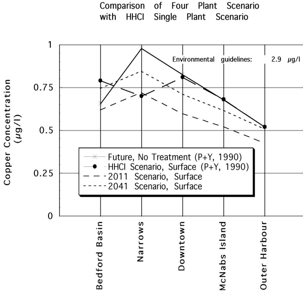
Figure 2.4 Predicted Copper levels - comparison of four plant and older one plant results.
