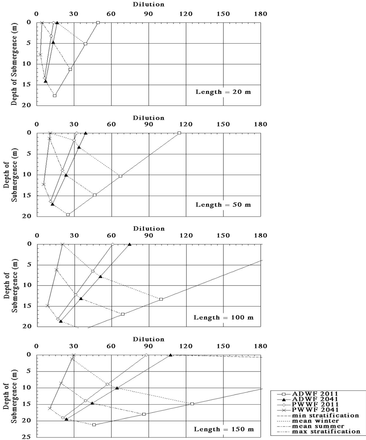
Figure 4.8 Diffuser analysis results - Site 4b.
