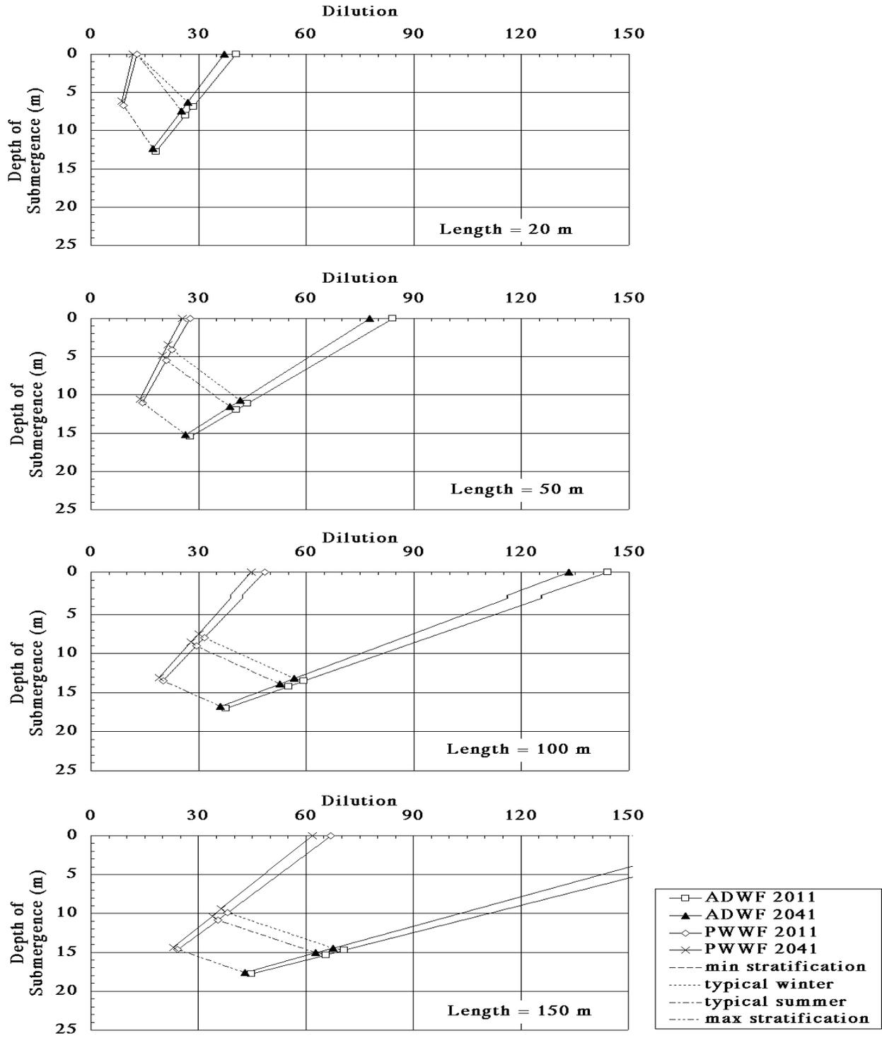
Figure 4.2 Diffuser analysis results - Site 1b.
