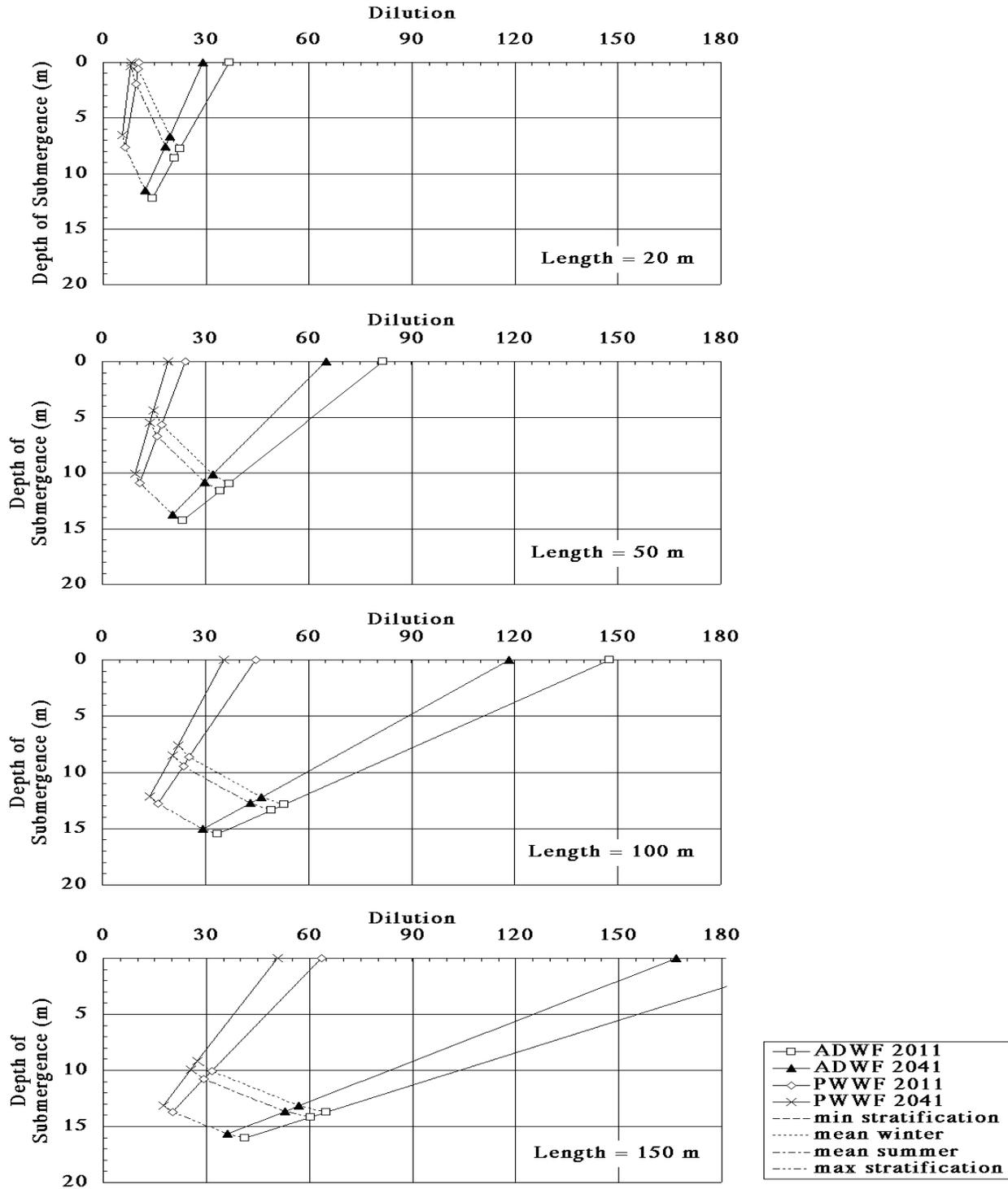
Figure 4.6 Diffuser analysis results - Site 3b.
