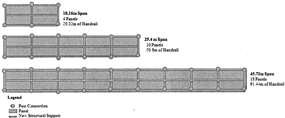
Analysis indicated that although this alignment allows for the re-use of existing handrail connections, it would require a significant amount of additional structural support and new material. New structural support would be required in the longitudinal and transverse directions in order to properly support the sidewalk deck panels.
