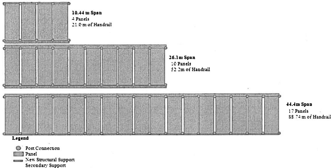
In this alignment, the sidewalk deck panel kick plate would need to be removed in order to ensure a flat travelling surface. Similar to Alignment A, new structural support will be required, though for Alignment B it will largely be located in the longitudinal direction of the structure with interim secondary support to pick up the free edge of each sidewalk panel.
