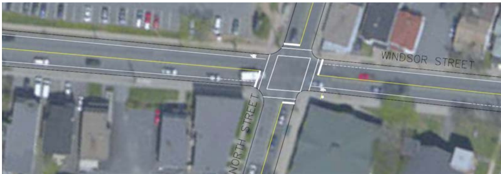
Figure 5.2 Bike Lanes maintained at intersections (Option A)
