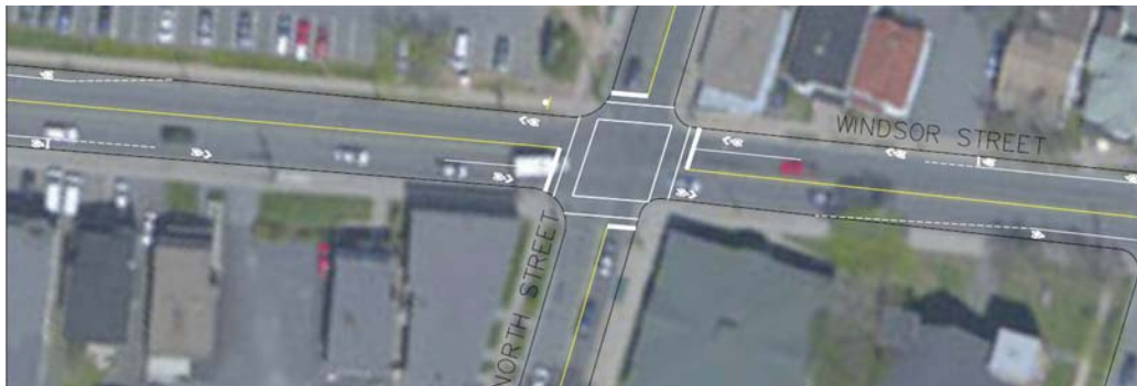
Figure 5.3 Bike Lanes discontinued at intersection approaches with shared lane (Option B)
