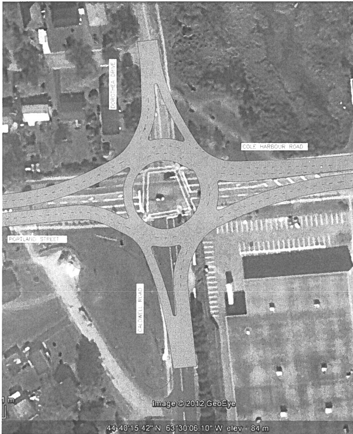
Figure 8 Potential Portland Street at Caldwell Road Roundabout
