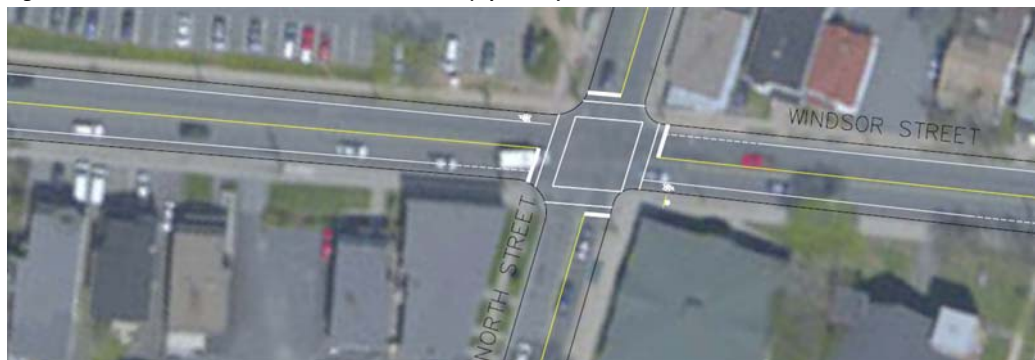
Figure 5.2 Bike Lanes maintained at intersections (Option A)
