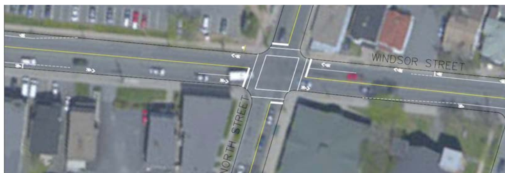
Figure 5.3 Bike Lanes discontinued at intersection approaches with shared lane (Option B)
