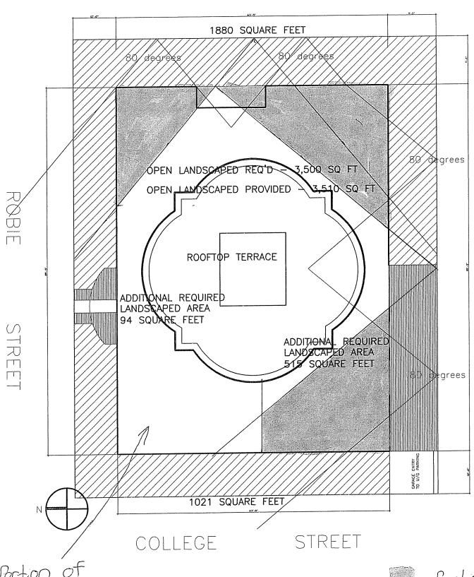
Portion of building that SITE & ROOF PLAN scale: 1/8" = 1'-0"
