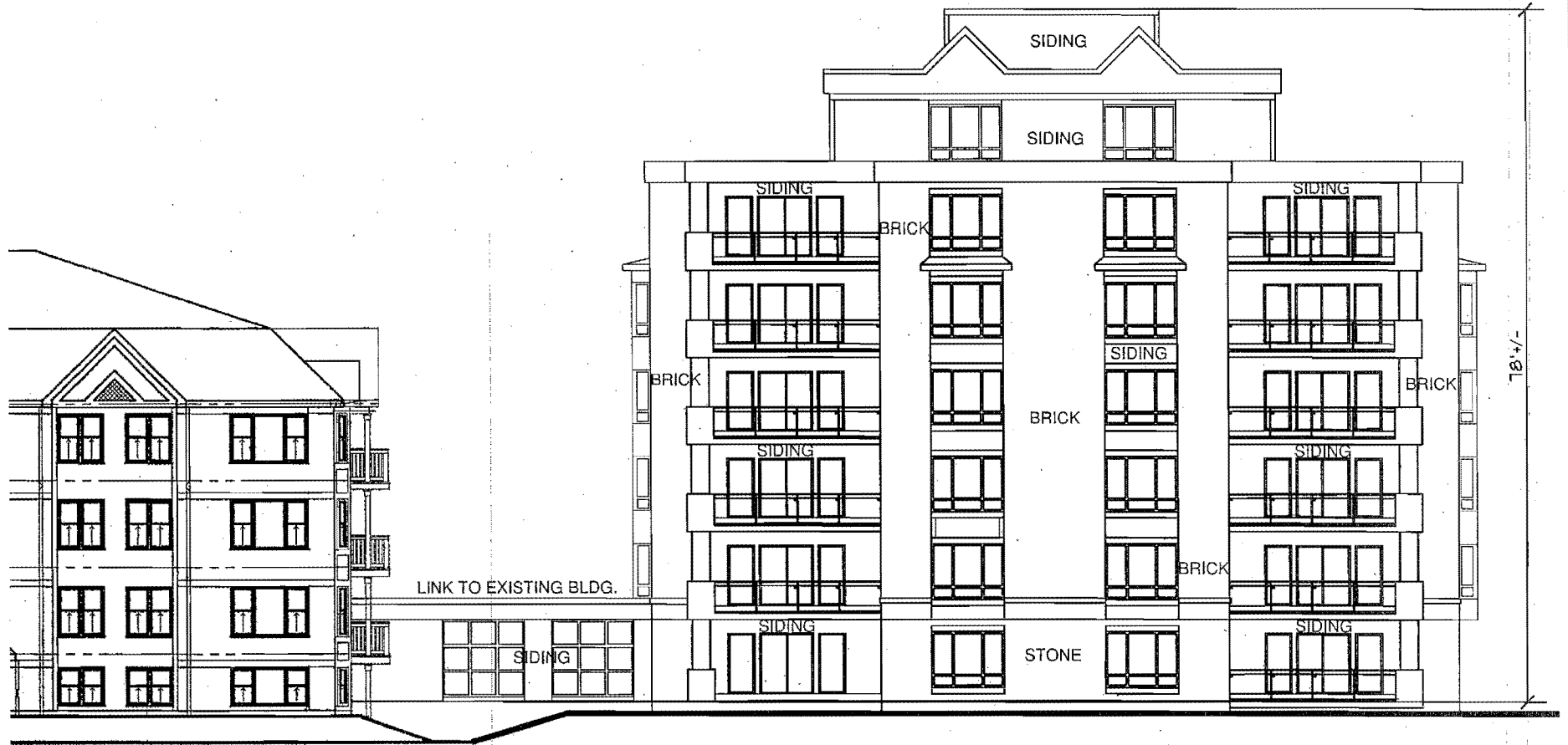
ADDITION - REAR ELEVATION "C" (NORTH)
