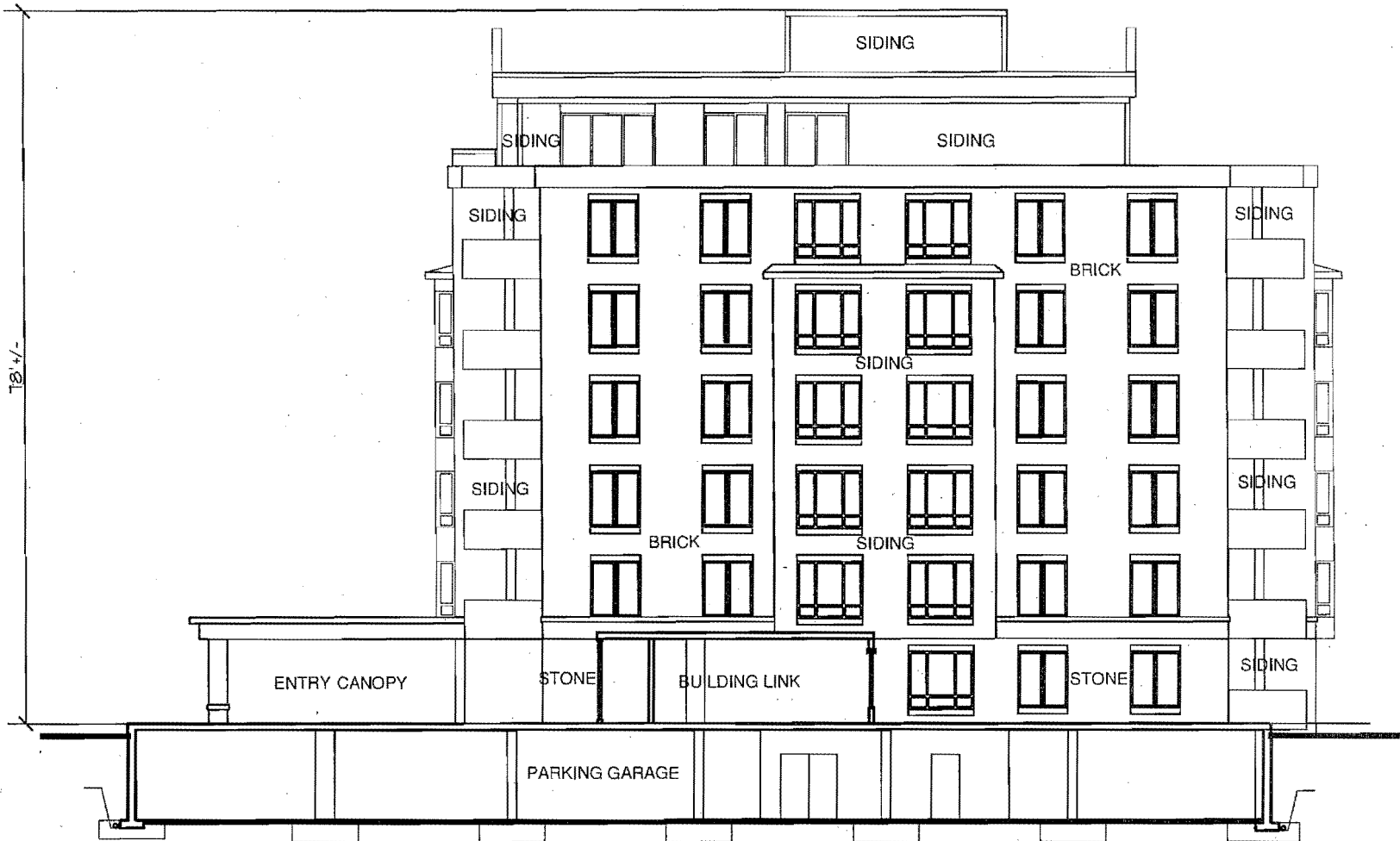
ADDITION - BLDG LINK ELEVATION "D" (EAST)
