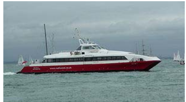
Exhibit 6: Red Funnel 38 knot 190 Passenger Vessel
