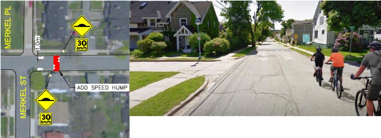
Figure 4.3: Concept for use of speed humps for traffic calming on local street bikeway.
