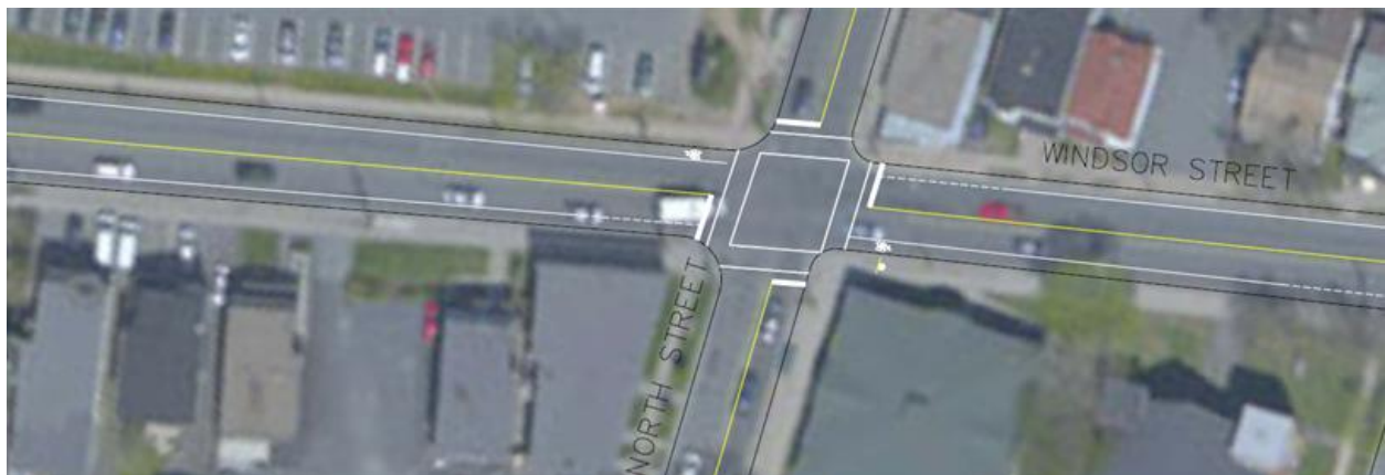
Figure 5.2 Bike Lanes maintained at intersections (Option A)
