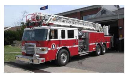
A Quint is capable of performing multiple tasks (pump, water tank, fire hose, aerial device, and ground ladders) with each of these functions making up one of its five (Quint) capabilities.
