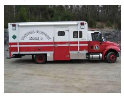
Tactical support trucks carry specialized equipment to the incident scene such as additional breathing apparatus air tanks and HAZMAT equipment.
