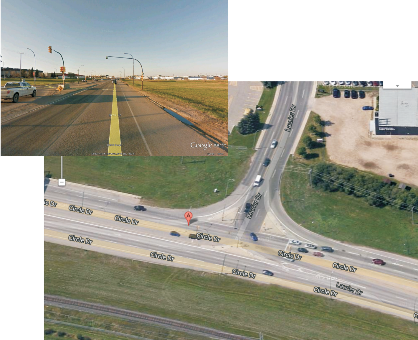
In this example intersection in Saskatoon, SK uses a large concrete island and a painted cross-hatched area to create a separation.
