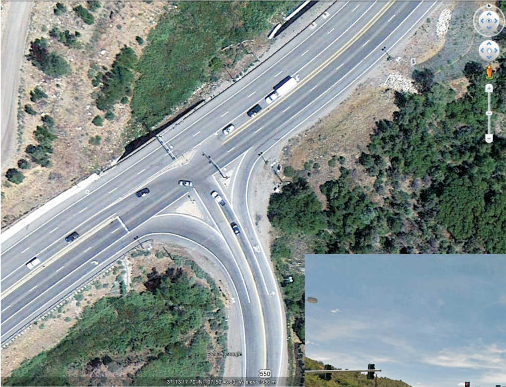
This example intersection near Durango, CO uses delineator posts to separate the left turning traffic from through traffic.
