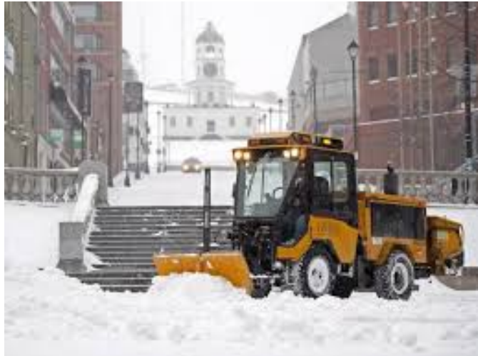
Figure 5-3 Sidewalk Clearing with Articulated Tractor in Downtown Halifax
